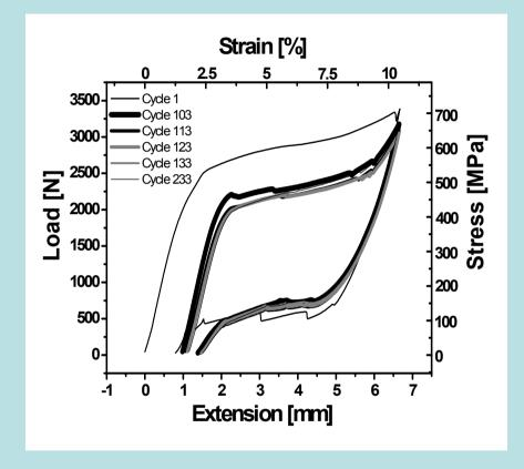
Recovery of 2.46 mm diameter NiTi wire by heating to 100°C. Cycle 1 compared with the cycles after thermal treatments to 100°C: cycles 103 (first recovery), 113 (second recovery), 123 (third recovery), 133 (fourth recovery), 233 (fifth recovery). The cycles after heat treatment to 100°C result very similar among them
