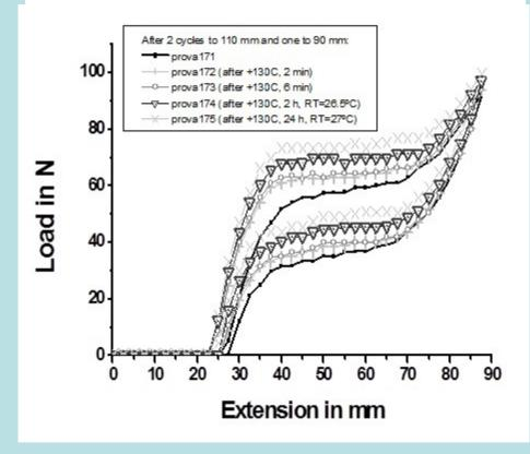
overstrained 1m long, 0.5 mm diameter NiTi wire. An as furnished wire was subjected to 2 cycles to 11% and one to 9%, and then followed the represented cycles: one cycle (prova171) to 8.75%, 2 min at 130°C, one cycle to 8.75%, 6 min at 130°C, one cycle to 8.75%, 2 hour at 130°C, one cycle to 8.75%, 24 h at 130°C and one cycle to 8.75% (prova175).
