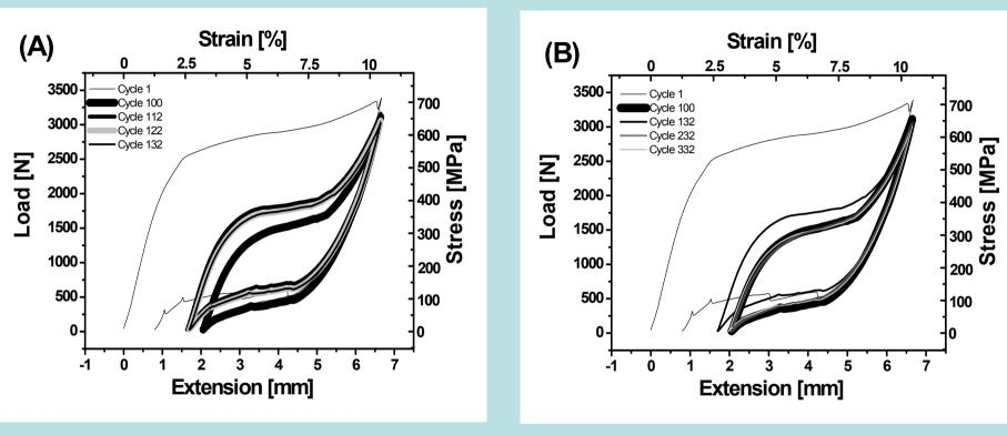
Cycling effect on 2.46 mm diameter NiTi wire. (A): Cycles 1, 100 (at the end of ontinuous cycling), 112 (10 cycles more after first heat treatment), 122 (10 cycles more fter second heat treatment), 132 (10 cycles more after third heat treatment). (B): Cycle 1, 100, 132, 232 (100 cycles more after fourth heat treatment), 332 (100 cycles more after fifth heat treatment).
