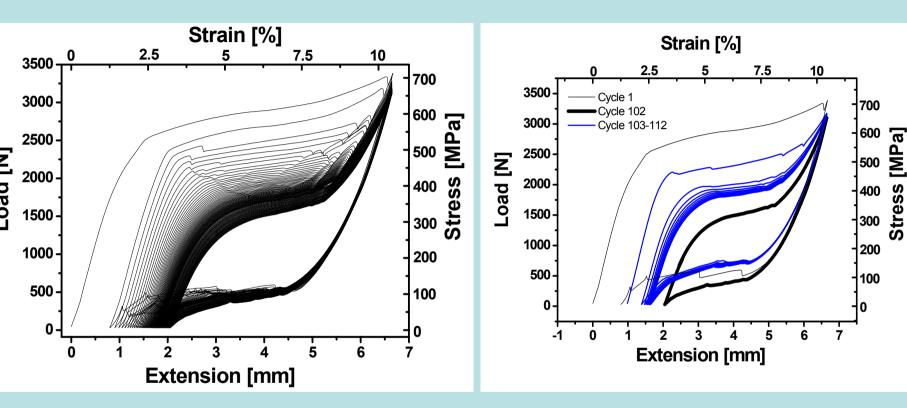
Recovery effect on 2.46 mm diameter NiTi wire. Left, first 100 cycles. Right, Cycles 1, 102 done after 5 h at room temperature once finished the first 100 cycles, and cycles 103-112 after heating to 100°C for 3.5 h.
