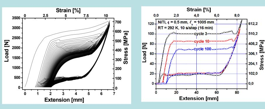
Cycling effect: Left: 2.46 mm diameter NiTi wire. Cycles 1 to 100. The first cycle includes some gripping effects from the mechanical testing machine.
