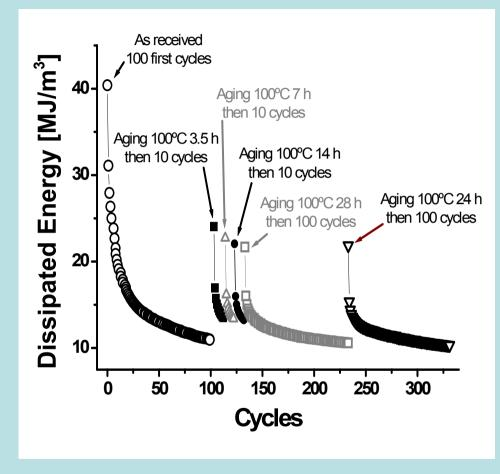
Specific dissipated energy per cycle. Recovery with thermal treatment to 100°C on 2.40 mm diameter NiTi wire.
