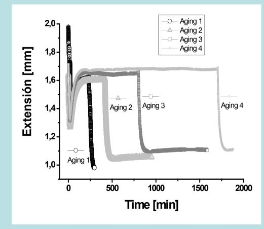
Extension as a function of time during the thermal treatment of NiTi wire 2.46 mm diameter, at 100°C, for different recoveries.
