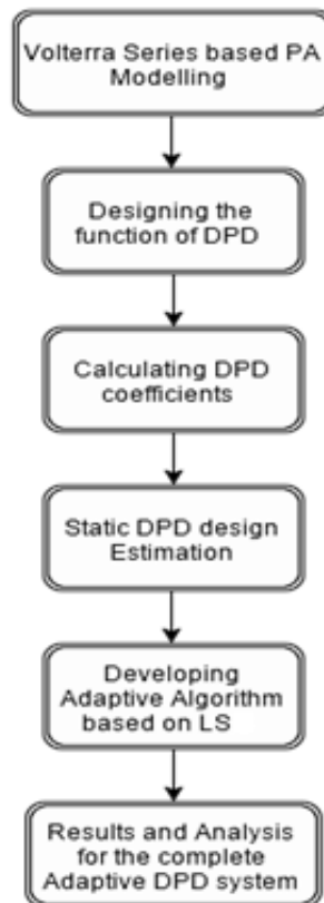
Figure 26: Flow diagram of DPD implementation phase
