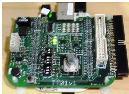
Fig 6.5: LED LD1 in cape TT01v1 switched on, corresponding to app GPIO1
