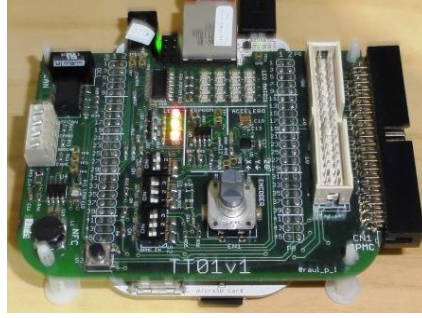
Fig 6.6: LEDs LD1, LD2 and LD3 in cape TT01v1 switched on, corresponding to app GPIO2
