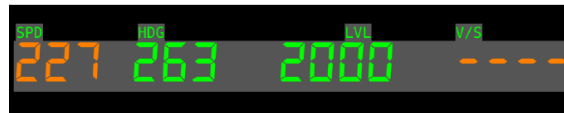
Figure 2.3: CAS (kt), Altitude (ft), Heading ( ^{\circ} ) and Vertical Speed (ft/min) indications on the HMI
