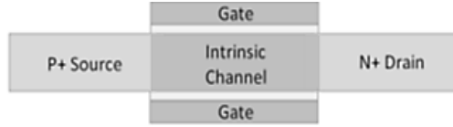
Fig. 1 Double-gate n-TFET structure
