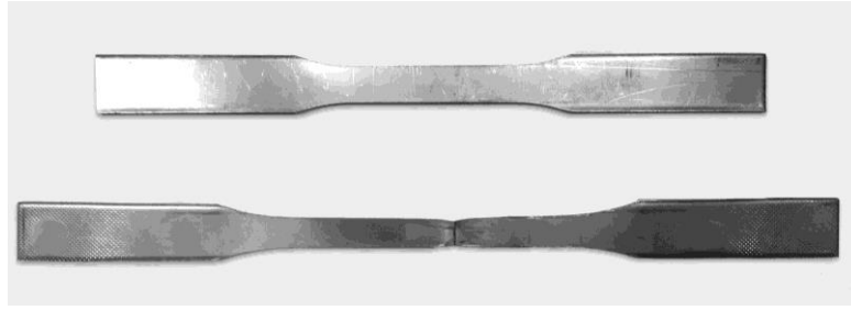
Figure 2. Austenitic stainless steel coupons before and after testing.
