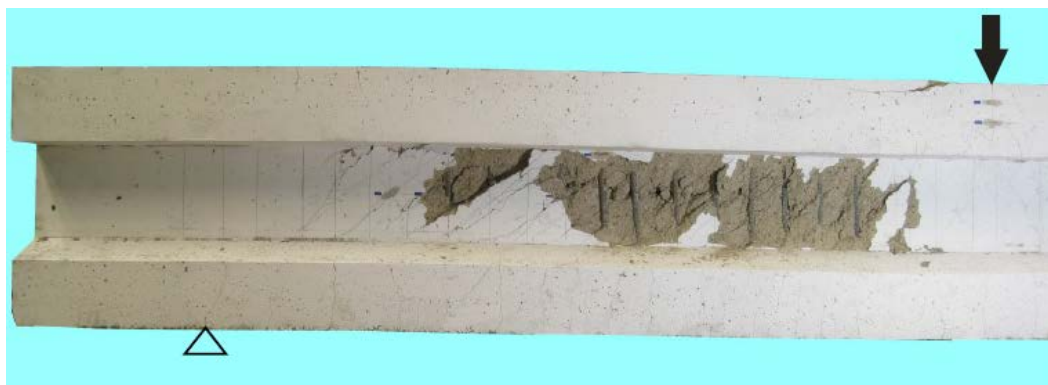
Figure 24: Cracking at failure in experimental S2AN-2.3-4 ( \rho_w = 2.26\% , f_{cm} = 33.5 \text{ N/mm}^2 )(Kurth 2012)
