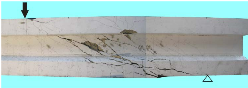
Figure 20: Cracking at failure in experimental S4AH-0.8-7 ( r_w = 0.75\% , f_{cm} = 42.2 \text{ N/mm}^2 ) (Kurth 2012)
