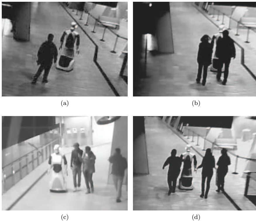
Fig. 6: Group spatial arrangements: (a) guide-visitor couple with leader-follower formation; (b) guide-visitors triple in a leader-follower spatial arrangement with robot heading the group followed by a dyad; (c) guide-visitors triple with V-like pattern; and, (d) four-agents with robot leader followed by a triad.
