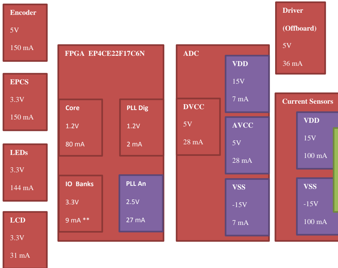
Figure 42. System power requirements.
