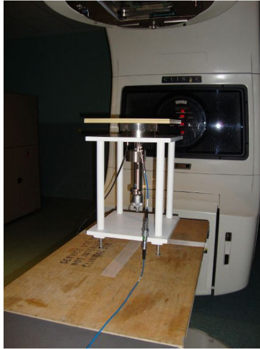
Figure 4.1: Experimental setup used for the measurements in the build-up region with the Extrapolation Chamber.
