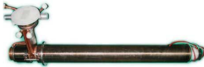
Figure 2.1. 9 MeV standing wave electron linac for industrial applications [10].
