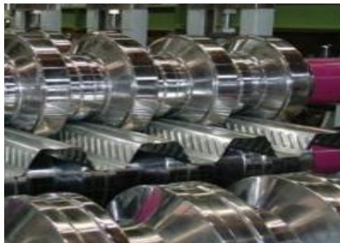
Figure 4 Steel sheeting conformation.[7]
