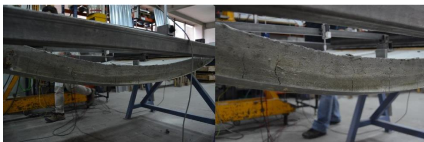
Figure 36 Cracking on slabs
