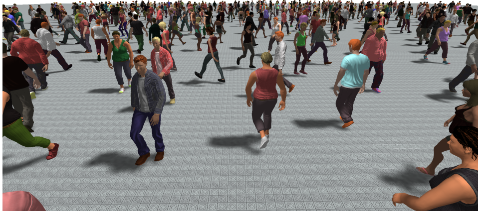
Figure 3.8: Scene where the closest agents are rendered as high detailed polygonal meshes and the One Textured Quad Impostor is used for the furthest away characters
