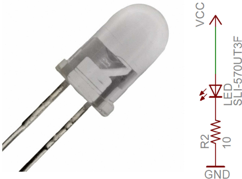
Figure 12: Red LED picture and circuit schematic
