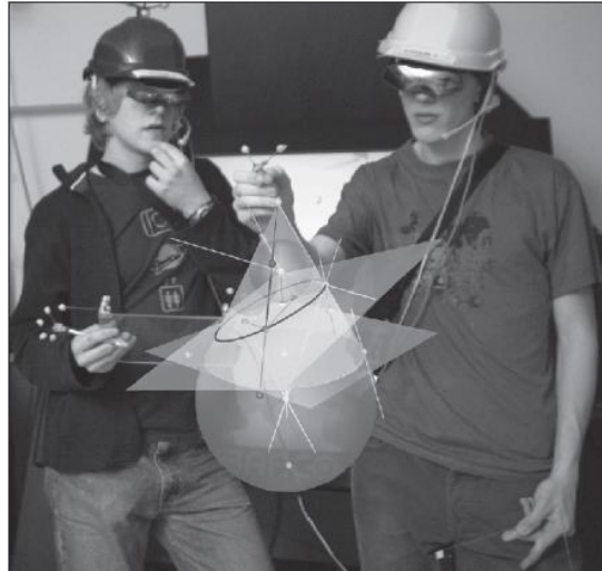
FIG. 21. Augmented reality system with marked objects and HMD displays. Reproduced from Lee (2012)
