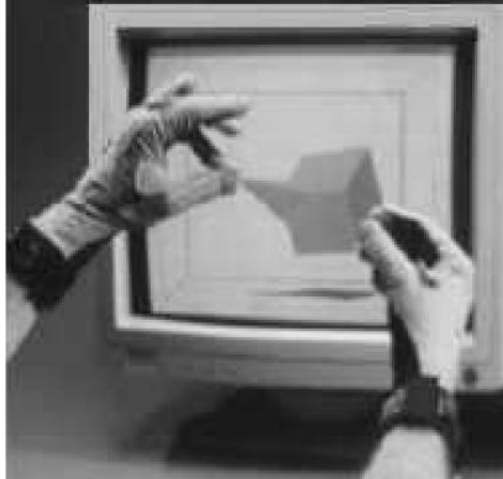
FIG. 22. A virtual object manipulated using data gloves. Reproduced from Sala & Sala (2005)
