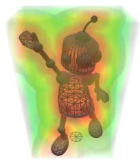
Figure 3.3: Distance field that shows the distance to the surface of a 3D model.
