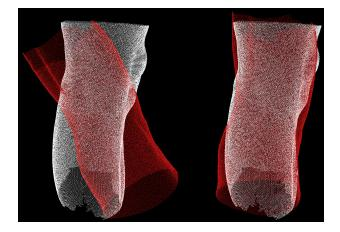
Figure 8.15: In the left, knee in red rotated 150 degrees about the X axis. In the right, the knee after the ICP alignment process.
