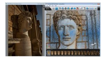
Figure 3.6: 123D Catch in action. In the left, picture of the object. In the right, 3D model reconstructed using pictures.
