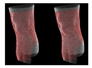
Figure 8.4: Picture in the right shows the alignment of two knees belonging to the same person done using the ICP algorithm provided by the *Point Cloud Library*. Left picture shows the initial alignment.
