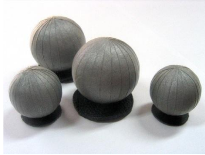
Figure 2.3.1 Passive markers [ www.qualisys.com ]
