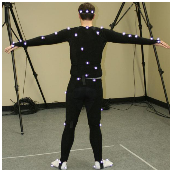
Figure 2.3.2 Active Markers [ www.sfdm.scad.edu ]
