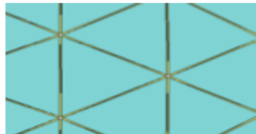
Figure 17: Scheme depicting the concept of finite element with high aspect ratio (left) and interface elements inserted within the mesh.
