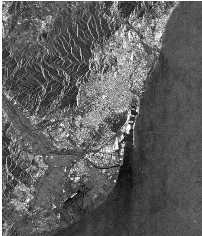
Figure 3.7: Region of the averaged module of an ERS SLC from the area of Barcelona. It shows the reflectivity of the scene. The city has a higher reflectivity (white), while the sea and the forests has a lower reflectivity (black). It is presented with a multilook of 5 \times 25 , that is, a spatial averaging of 5 samples and of 25 lines.
