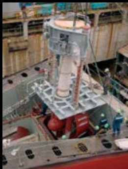
Wärtsilä retractable steerable thruster.
