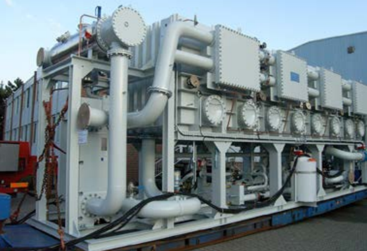
Wärtsilä Serck Como Thermal Desalinations Plants with Multi-Stage-Flash technology.
