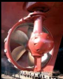
Wärtsilä modular steerable thruster.
