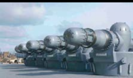
Wärtsilä underwater demountable steerable thrusters.
