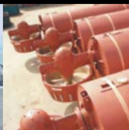
Wärtsilä containerised steerable thrusters.
