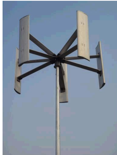
Vertical Axis Wind Turbine [6]
