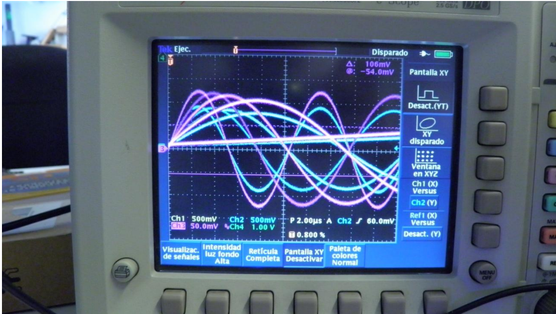
Figure 5.2: D/A output and A/D input signals on oscilloscope
