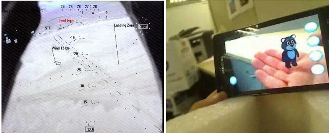
(a) NASA X38 display showing video map overlays including runways and obstacles during flight test in 2000.
