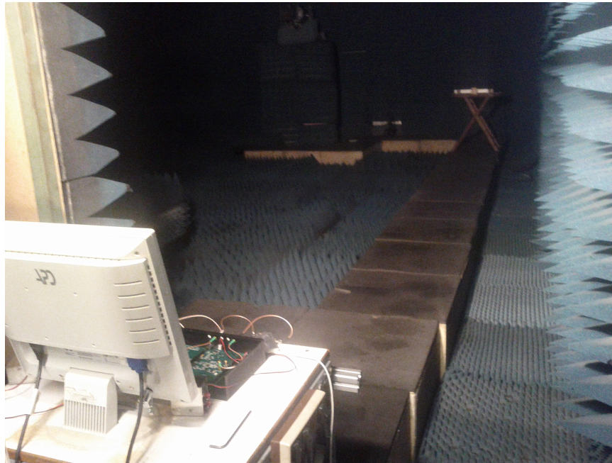
Figure 3-8: Measurement system validation in the anechoic chamber.
