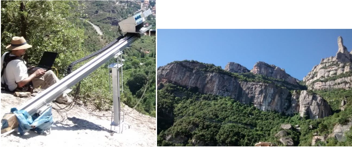
Figure 4 - 11 Left: X-band UPC GBSAR system mounted in the Montserrat test site. Right: Illuminated scene in the Montserrat test site.
