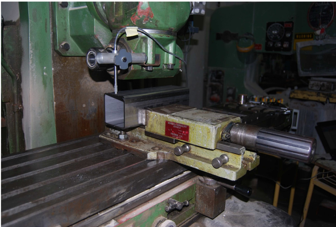
Figure 51. Stub-column's imperfection measurement
