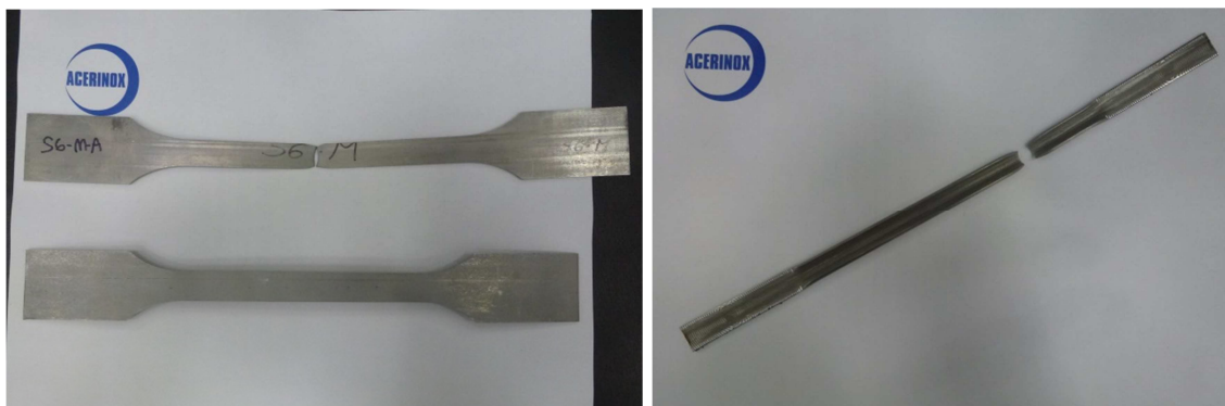
Figure 47. Typical failure modes for flat and corner coupons after testing.
