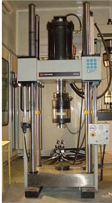
Figure 56. INSTRON 8805 testing machine
