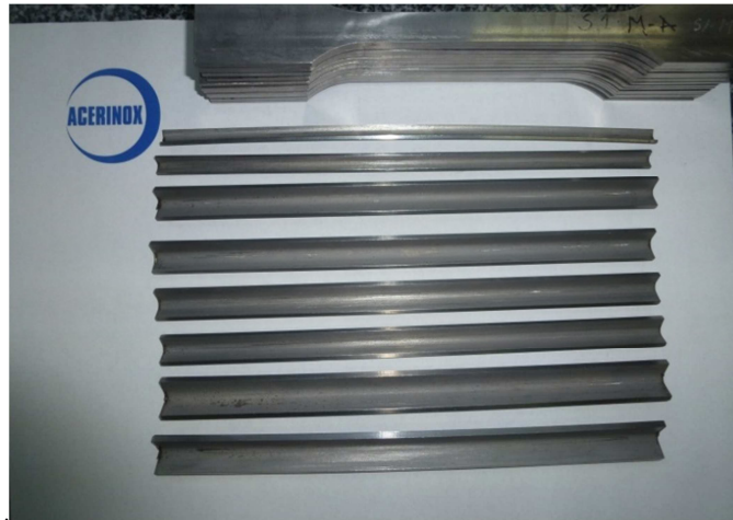
Figure 45. Tensile coupon specimens: necked flat coupons and straight corner coupons
