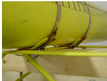
b) Jubilee clips around pontoon body
