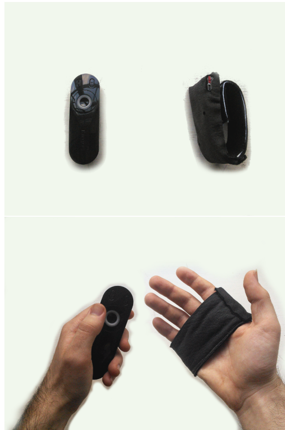
Figure 6: A one-button controller, on the left, and a haptic glove, on the right
