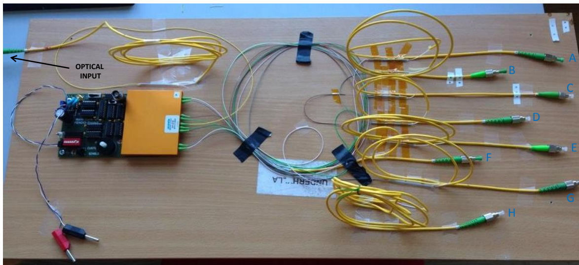
Figure 6.4. Test board with Sercalo SW1X8 and connectors at the outputs A-H
