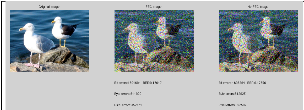
Figure 4.9.1. FEC + 8b/10b model working with a SNR of 5dB.
