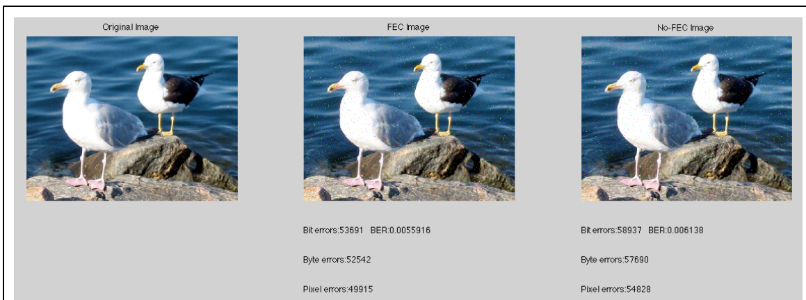
Figure 4.5. System with only FEC working with a SNR of 7dB.
