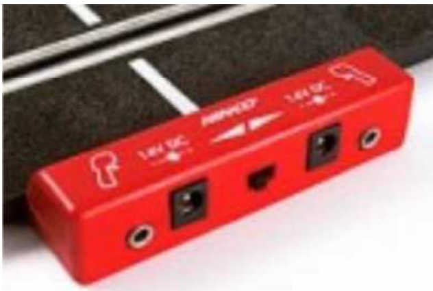
Fig. 4. Panel racetrack connections
