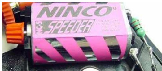
Fig. 9. Nc-5 speed motor with 22 ohms resistance
