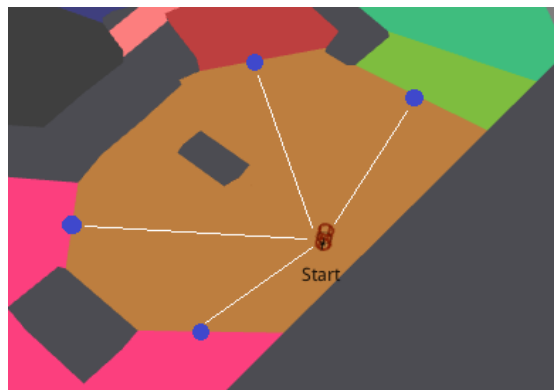
FIGURE 3.13: Connect Start node to the graph: Red circles are portals of the orange partition. White lines are the computed intraedges. Gray polygons are obstacles or no walkable areas.
