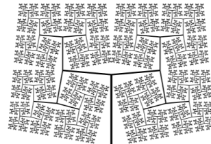
Figure 2.12: Binary tree generated from a parametric L-system with a single production rule A(s) ::= F(s)[+A(s/R)][-A(s/R)] applied 10 times to the axiom \omega = A(1) . \delta = 85^\circ , R = 1.456 . Image from [14].
