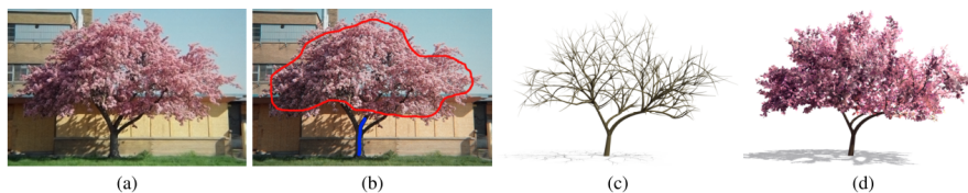
Figure 2.20: Tan et al. single image method overview: input image (a), user-drawn strokes (b) for crown (red) and branches (blue), generated branch structure (c) and final tree model (d). Image from [51].
