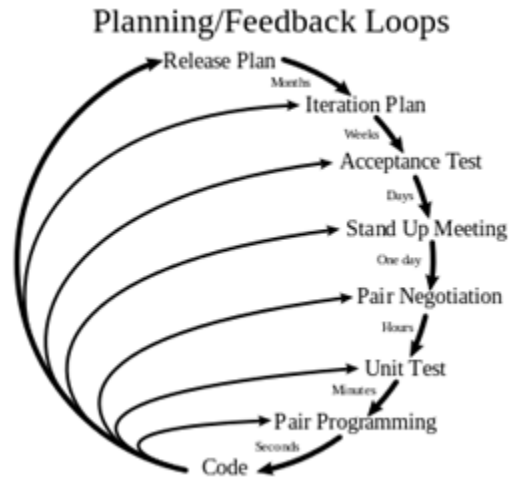
Figure 7.1: Planning and feedback loops in extreme programming
