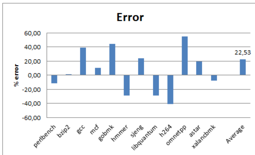
Figure 5.11: Relative error with out-of-order processor model (reg=12 & window=15)
