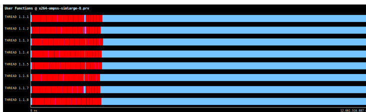
Figure 7.1: Trace file showing Tasks executed within OmpSs version with simlarge as input set and running on 8 threads
