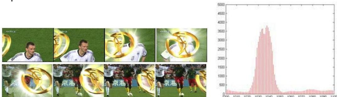
Fig. 2.7 Logo transition and Intensity mean square difference after applying the median filter
