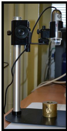
**Figura 5.19 Microscopio *Dino-Lite Optical Microscope Pro***
