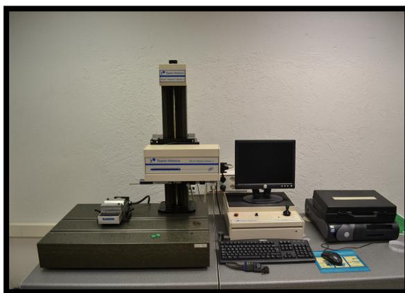
**Figura 5.11 Rugosímetro Taylor-Hobson Talysurf series 2**
