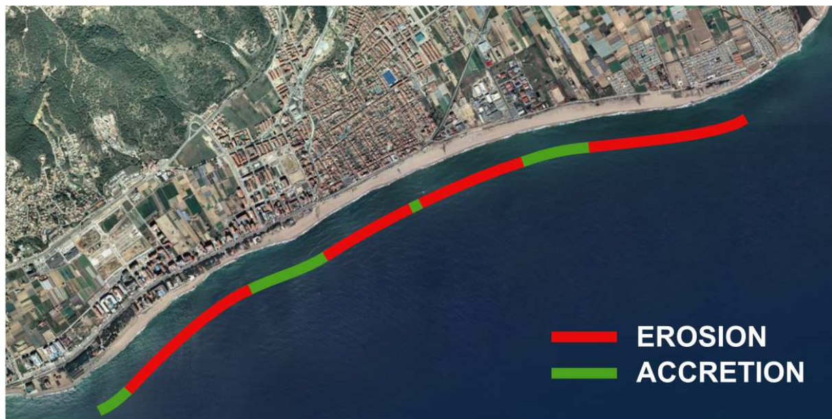
Figure 6.7. Spatial distribution of the areas of erosion and accretion along the beach of Malgrat (not considering the overwash of the backshore).
