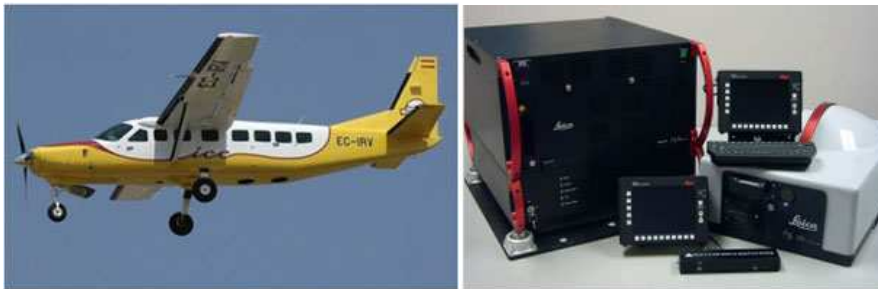
Figure 2.3. LIDAR at the ICC. Left: Cessna Caravan 208B, one of the planes used for the surveys; Right: LIDAR sensor LEICA ALS50 phase II (ICC).
