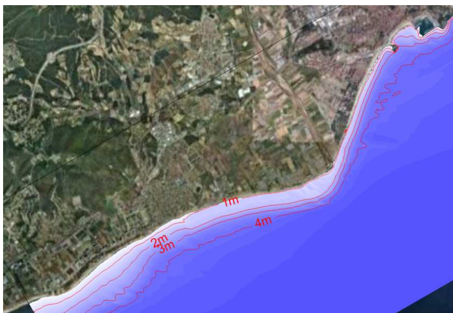
Figure 3.14. Propagated wave heights at the peak of the storm (26/12/2012, 18:00) using the mean period.
