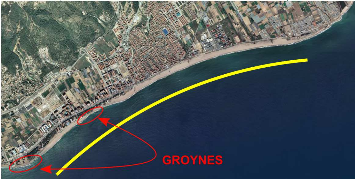
Figure 6.8. Irregularities in the beach of Malgrat: groynes and changing orientations.
