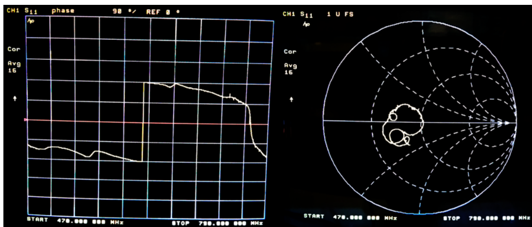
Figure 12: Measured reflection coefficient phase and Smith Cart (same band).
