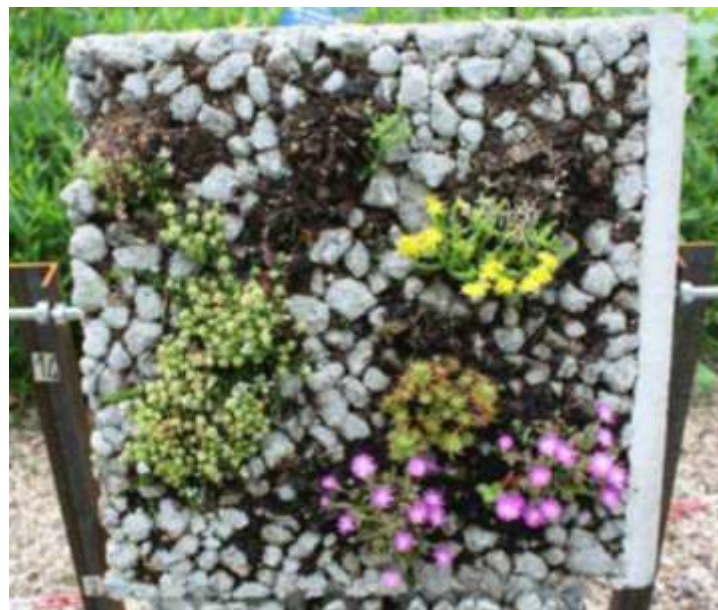
Figure 8. Concrete prefabricated panels with vegetation. (Ottelé 2011)
