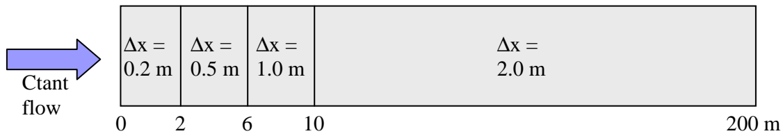
Figure 11 - Schematic diagram showing the dimensions and spatial discretization in the one-dimensional domain.
