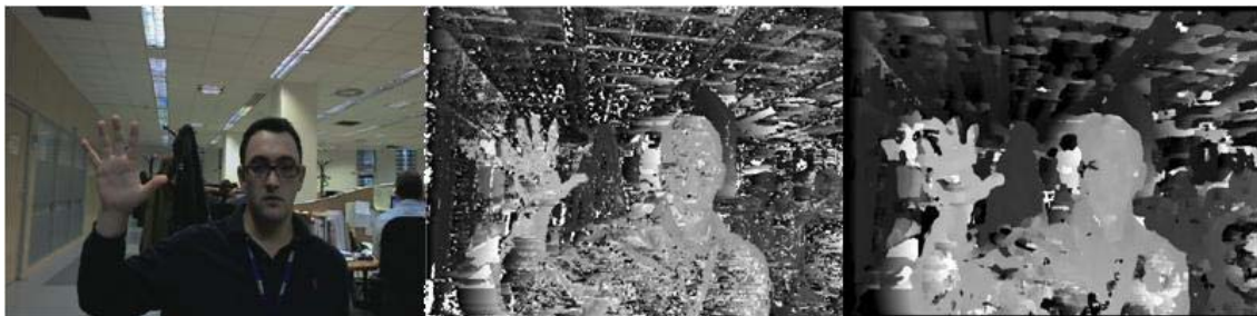
Fig. 2.5 Reference view and disparity maps window 5x5 and 15x15 with 80 disparity levels.
