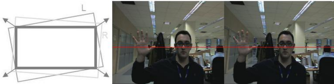
Fig. 2.3 Intersection, rectified and scaled images.
