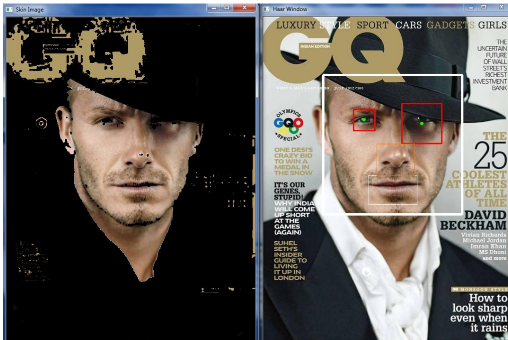
Fig. 3.7 Right eyes detection thanks to right face detection helped by skinDetector.
