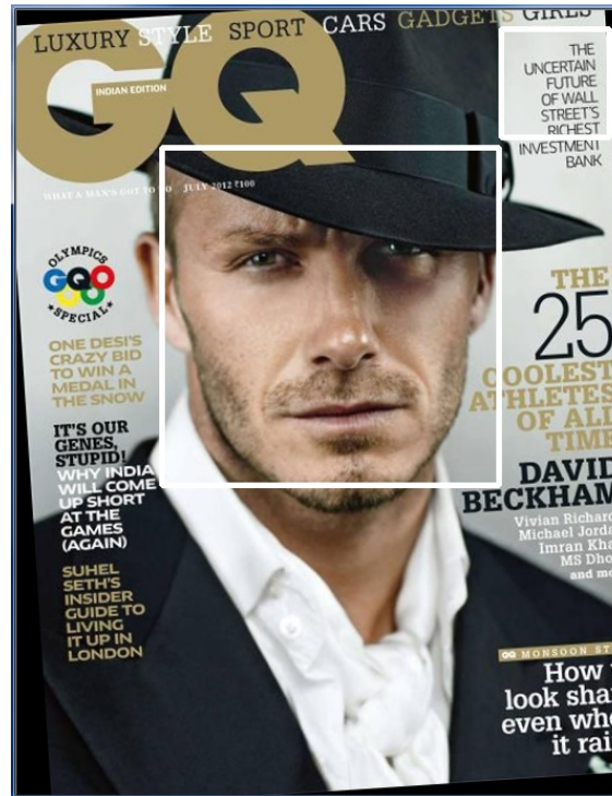
Fig. 3.6 False face detection in image. The false one will be discarded thanks to the skin detector.
