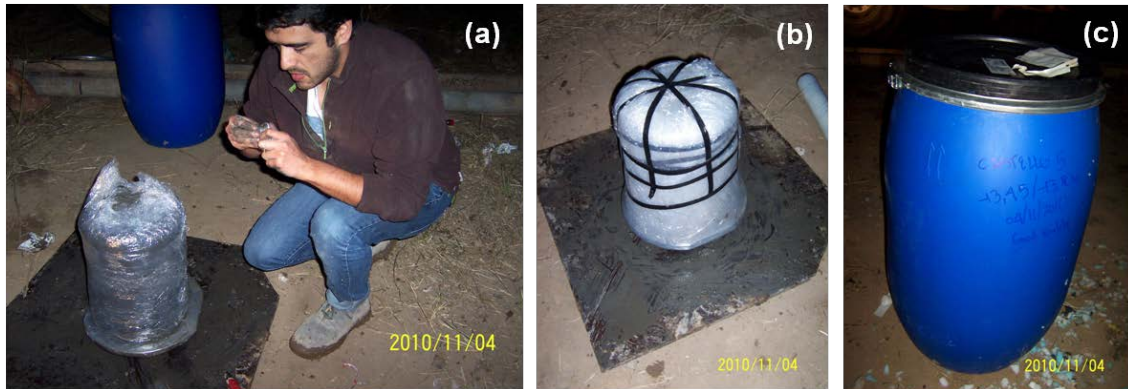
Figure 41. Covering and protection of the block samples.
