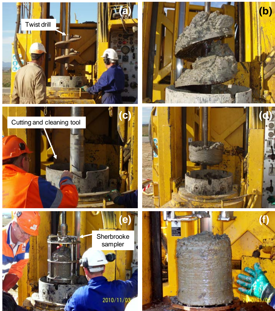
Figure 40. Sampling procedure using Sherbrooke sampler.
