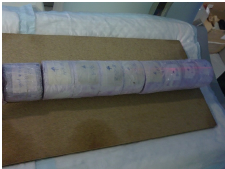
Figure 61. Placement of the calibration samples for the CT scan test.
