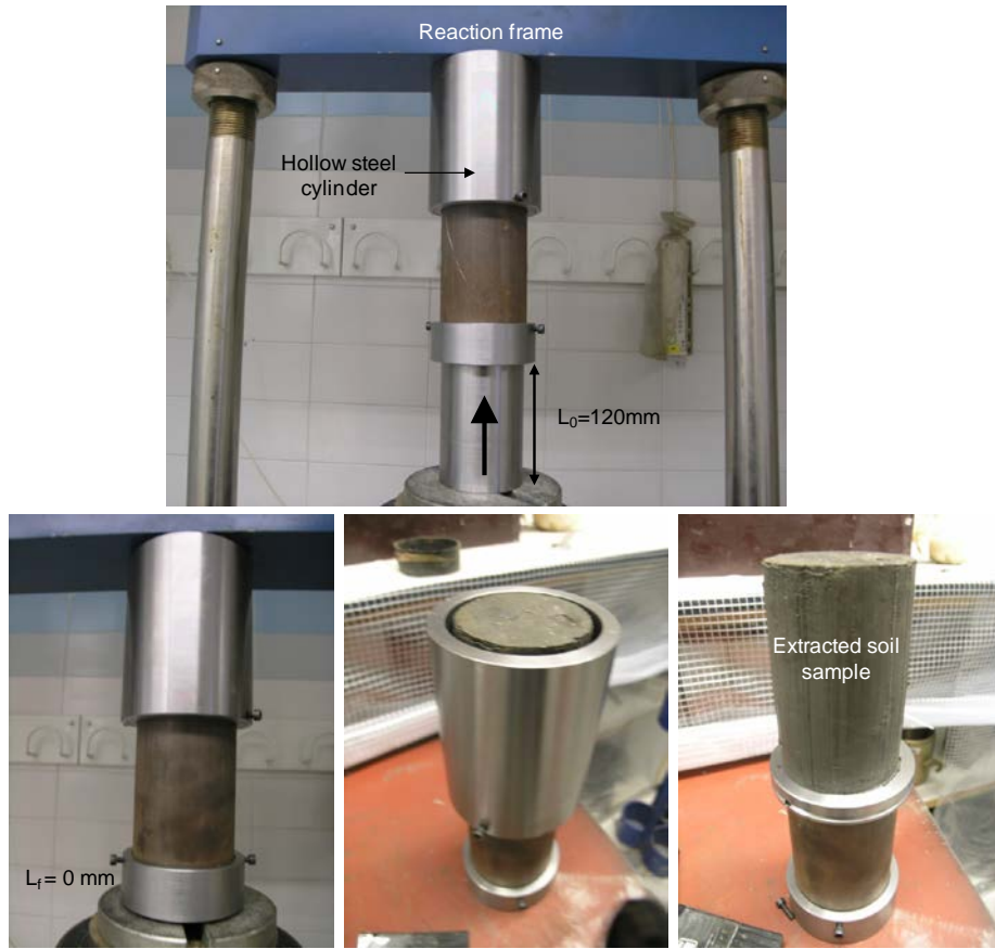
Figure 49. Extraction process of tube samples.
