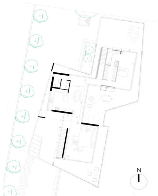
Image 2.1 Plan of the second floor of the housing
