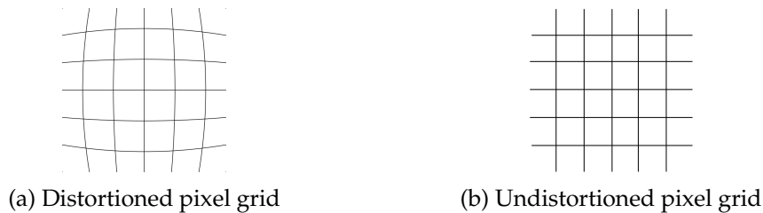
Figure 2.3.: Figure a) shows distorted pixel grid and b) shows the undistorted pixel grid. Lines have been mapped into curves by the non linear effect of the distortion.
