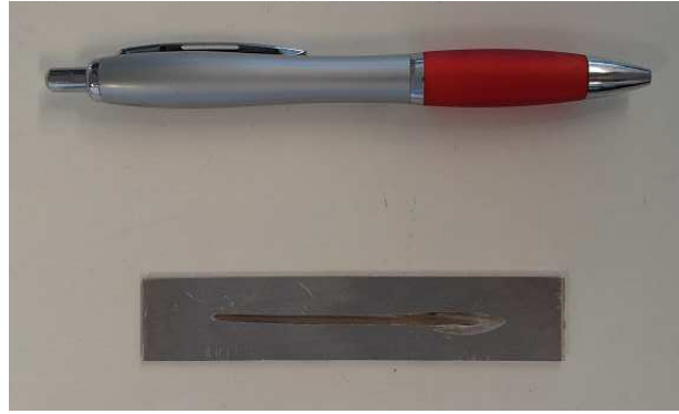
Figure 4.2: Test specimen with simulated crack.
