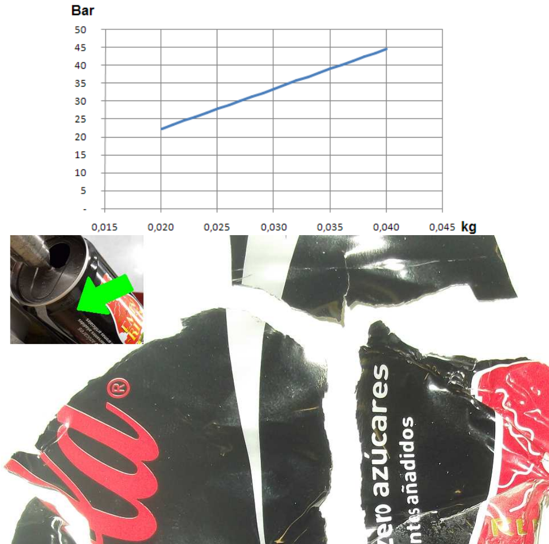
Figure 2 – (a) Max pressure vs Mass and (b) Crack propagation
