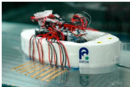
Figure 2 Robot actuated with 8 IPMCs to mimic rajiform swimming [31].
